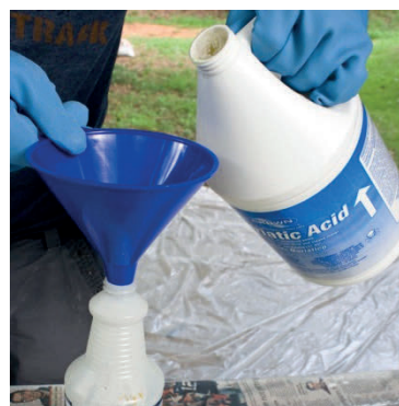
A worker is decanting a hazardous product from a larger container into a smaller, portable container
